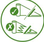
Ensure that the blade of the balewrapper's cutting mechanism is maintained in order to ensure a clean film cut after wrapping and thus avoid long film tails.
