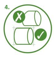
The baled material must always be evenly distributed over the width of the baler pick up. Bales should be dense and cylindrical in shape. The more compact the bale, the better the forage preservation will be.
