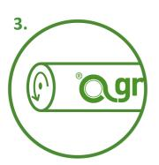
Reels should only be removed from protective packaging immediately prior to use. Open sleeve using the tear strip provided. The arrow on the reel end indicates the direction of wrapping.
