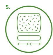
The Agribale reel must be placed centrally in the Intake unit so that the centre of the reel aligns with the middle of the bale.
